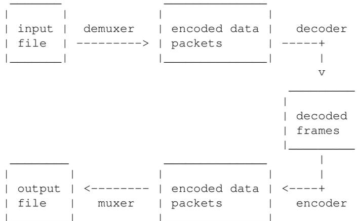
`ffmpeg` calls the `libavformat` library (containing demuxers) to read input files and get packets containing encoded data from them. When there are multiple input files, `ffmpeg` tries to keep them synchronized by tracking lowest timestamp on any active input stream.
