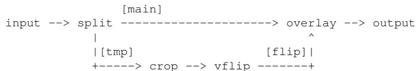
This filtergraph splits the input stream in two streams, then sends one stream through the crop filter and the vflip filter, before merging it back with the other stream by overlaying it on top. You can use the following command to achieve this:
