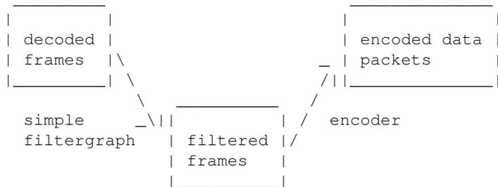
Simple filtergraphs are configured with the per-stream `-filter` option (with `-vf` and `-af` aliases for video and audio respectively). A simple filtergraph for video can look for example like this:
