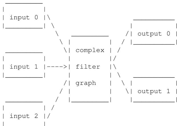
Complex filtergraphs are configured with the `-filter_complex` option. Note that this option is global, since a complex filtergraph, by its nature, cannot be unambiguously associated with a single stream or file.
